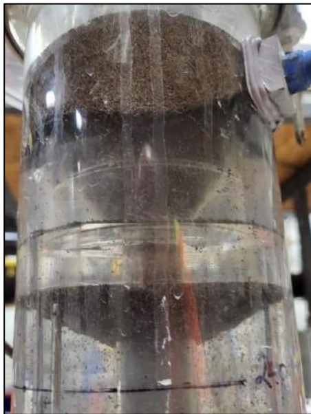
Figure 13-45: Photo of Zinc Thickening Test with Heavy Frothing of Overflow
