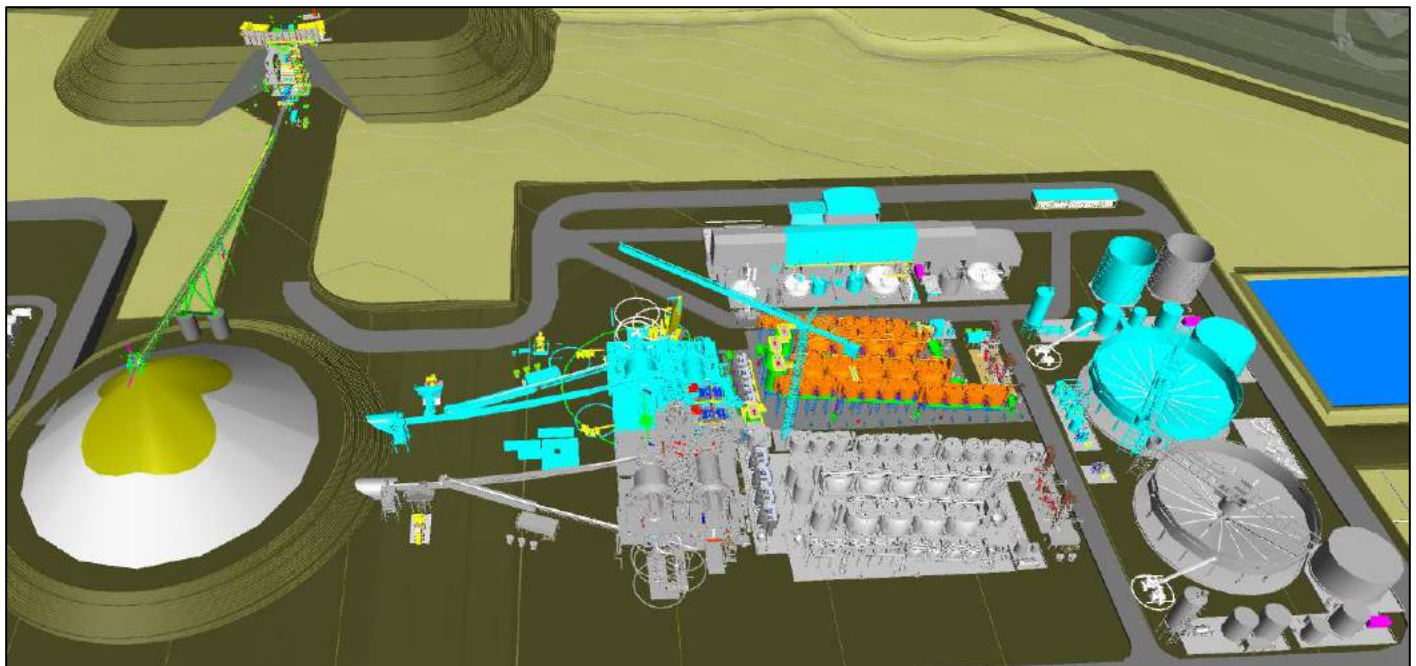
Figure 17-2: Overall Process Plant Layout
